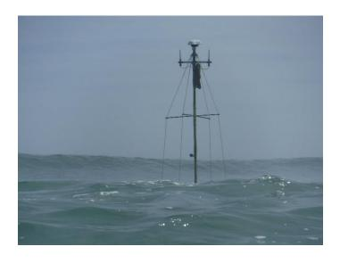
SurfROVer can be controlled via unpowered fiber umbilical or RF (with mast mounted antenna or antenna float system). Position monitoring can be achieved with either on-vehicle GPS (with mast, restricted to lower surf conditions and depths to 6 meters) or available INS capable of accuracies to 0.1 meter.
