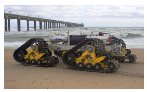
The low-profile design and wide footprint create an extremely stable vehicle for high energy environments and provides an excellent platform for deployment of a cable/pipeline tracker.
