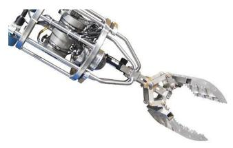
The Smart Grapple is suspended by a heavy lifting line which also controls its vertical motion. The later motion is provided by four vector configured thrusters. It has high intensity, dimmable LED lighting, a pan/orbit/zoom camera as well as a tooling camera integrated into the jaws.
