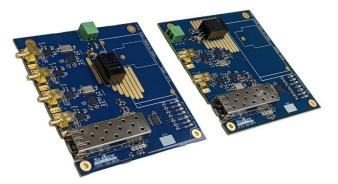
The HD-SDI converter may be stacked neatly on top of SeaView's other optical data cards; the fiber multiplexer and the Gbit Ethernet card. All data may be combined onto a single fiber via a compact wave division multiplexer (CWDM).
