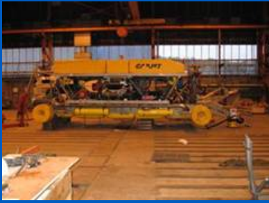
This is a shot of the 1 MegaWatt, 12m long, 14 Ton Capjet 650 being prepared to mobilize in Kristiansund, Norway. It is sitting in a ship building hanger. Probably the largest open building I have ever been in.
